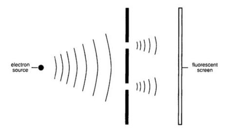
*Figure 14*. The double-slit experiment for electrons.
